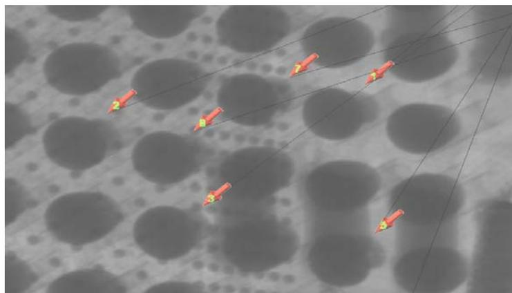
**Figure # 9: X ray images can detect HiP. Some HiP's are hard to catch. Inspector skills and tilt x- ray capabilities are needed**
