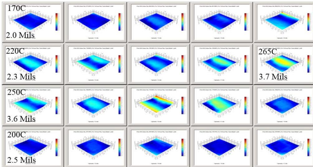
Figure # 16: Thermoire images at every 10 degrees showing BGA behavior under thermal stress
