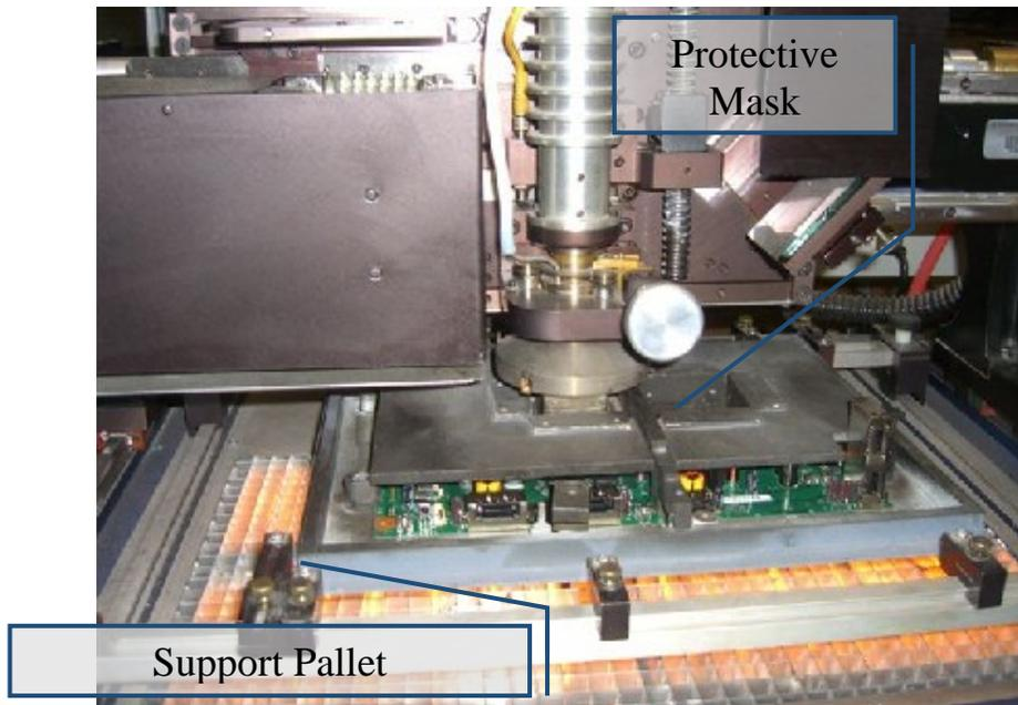
**Figure # 3: The BGA rework machine process:
