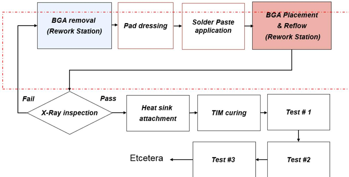
**Figure # 1: The BGA rework process:**
