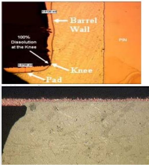
Figure 8. SAC305 solder can result in unacceptable copper dissolution in wave solder and surface mount (typically becomes an issue with rework).
