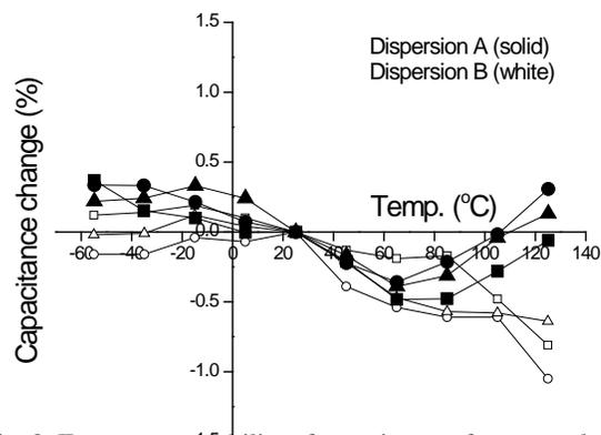
Fig. 3. Temperature stability of capacitance of two samples prepared by different suspension preparation routes
