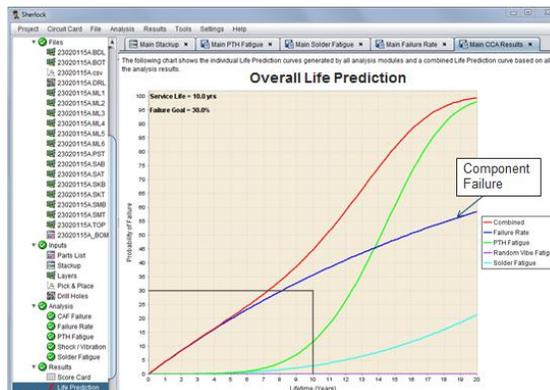
Figure 93. Life Prediction that combines component failure with PTH and solder fatigue.
