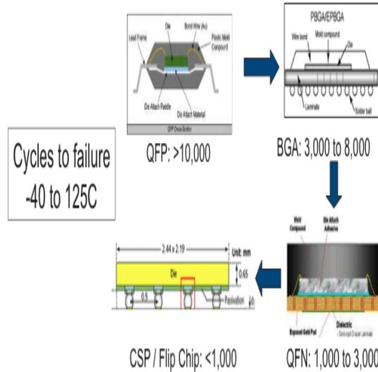
Figure 10. Cycles to Failure for Various Devices
