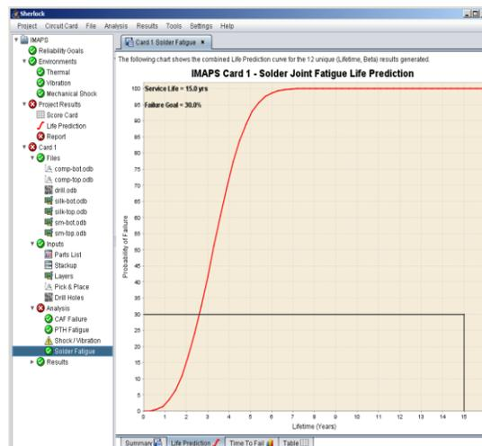
Figure 12 Solder Joint Fatigue Life Prediction (representing a very harsh underhood environment).
