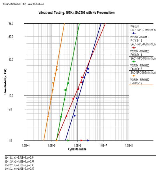
**Figure 56. Realistic High Cycle Fatigue Testing for SAC 305**
