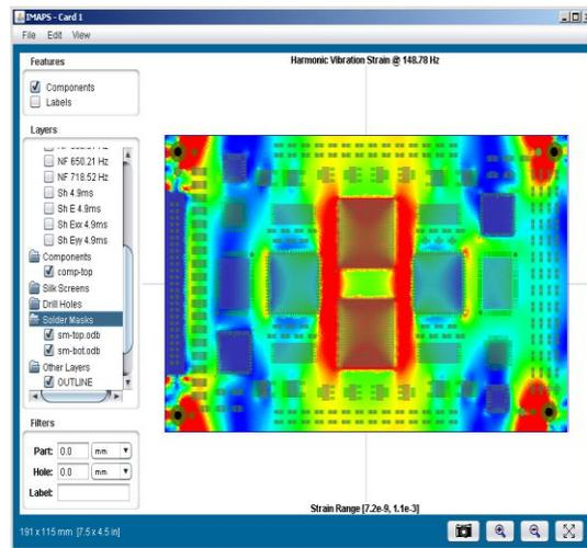
Figure 67 Graphical Vibration Results
