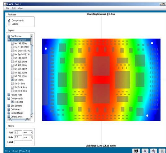
**Figure 20. Shock displacement results for a test board.**
