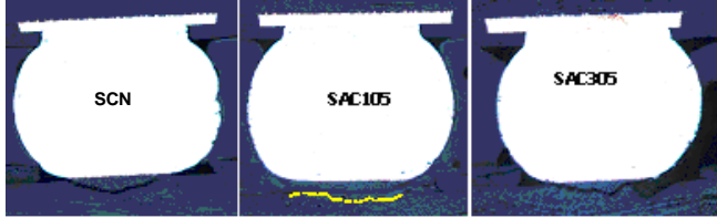
Figure 13. Pad cratering was seen on all samples.
