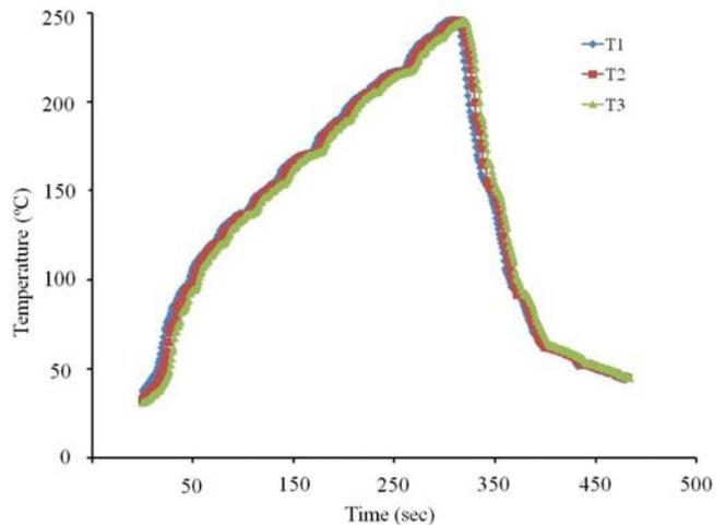
**Figure 3: Reflow profile for SAC305 solder paste**
