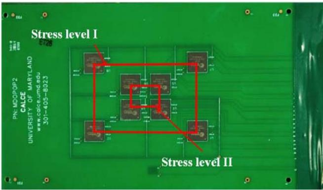
Figure 7: Stress levels under torsion on PWA
