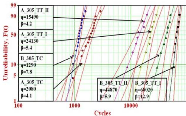
**Figure 11: Durability under torsion testing and thermal cycling for SAC305 packages**
