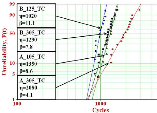
Figure 8: Durability under thermal cycling for test matrix
