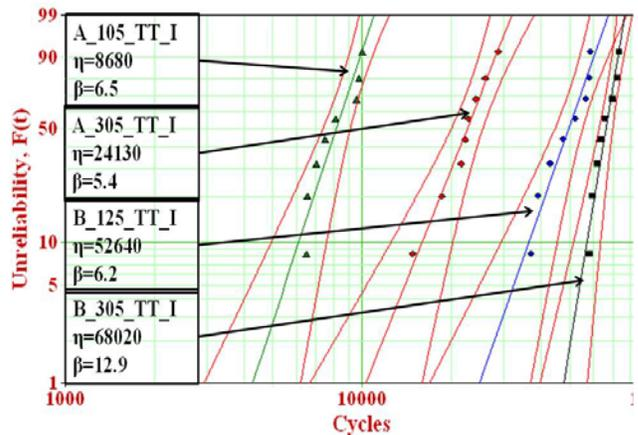
Figure 9: Durability under torsion testing for test matrix at stress level I
