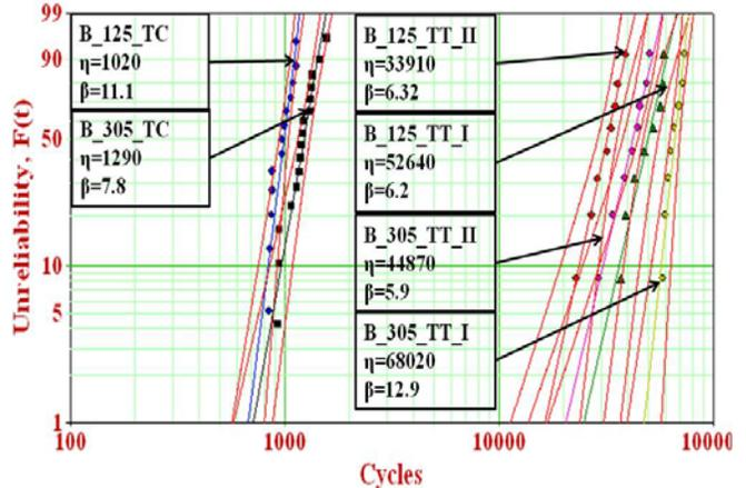
Figure 10: Durability under torsion testing and thermal cycling for type B packages
