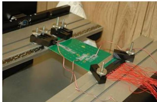
**Figure 6: Torsion test setup**
