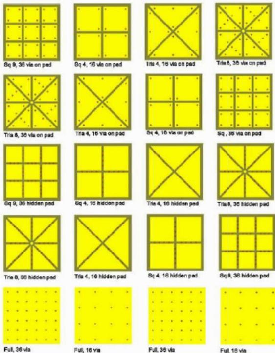
Figure 1. Pad design of the QFN test board showing thermal pad patterns<sup>1</sup>
