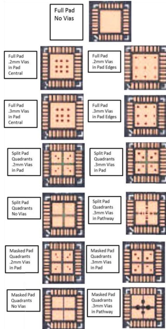
Figure 2. QFN thermal pad patterns tested
