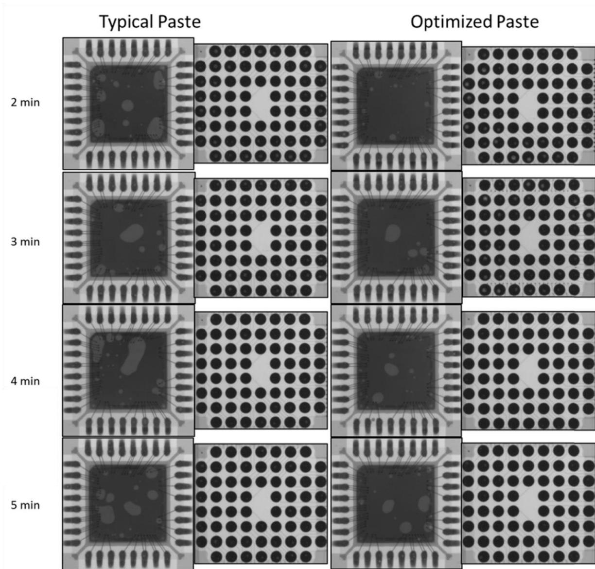
**Figure 4:** X-ray comparisons of reflow performance for QFNs and BGAs with a typical paste and a paste optimized to minimize QFN voiding
