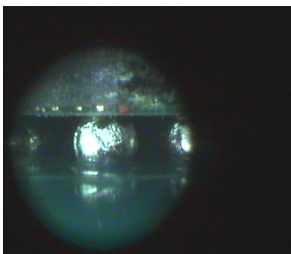
Figure 11: Good BGA ball and PLCC leads wetting in Vapor Phase soldering.
