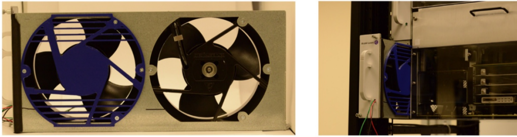
Figure 15 – Integrated guide vanes for local flow control at the fan exit
