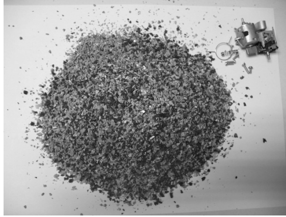
Figure 2: Sample Preparation - Grinding
