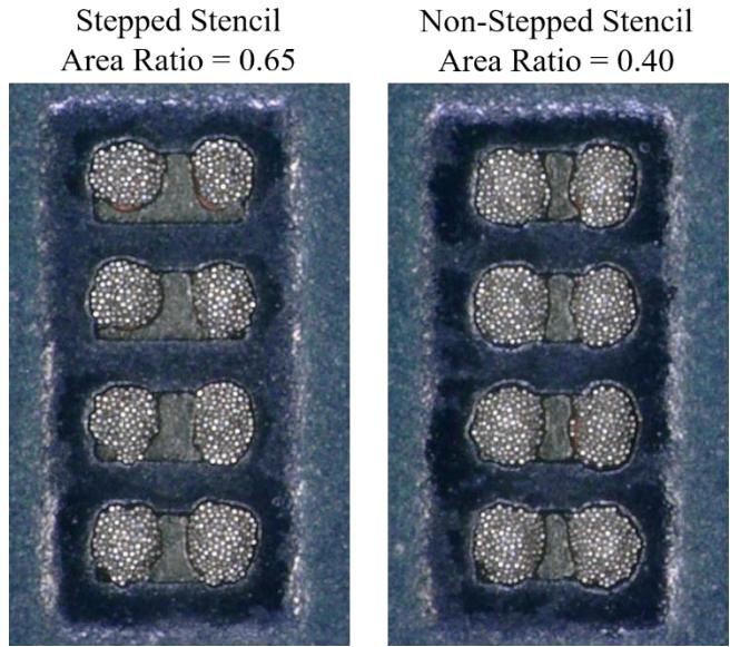
**Figure 3.** M0201 print deposits from the first assembly test comparing stepped and non-stepped stencil results.
