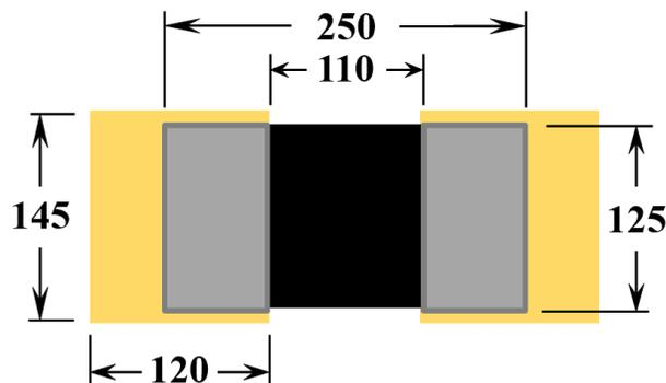
Figure 1. M0201 pad design (dimensions in microns).
