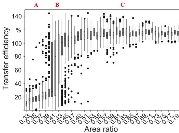
**Figure 8.** Solder paste print transfer efficiency scatter response to aperture area ratio per Rösch et al.[7]
