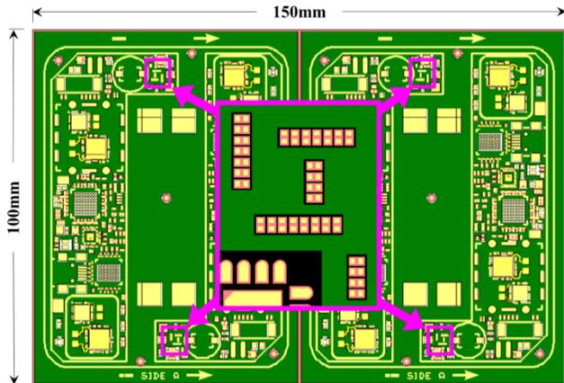
**Figure 2.** M0201 pad locations on test circuit board.
