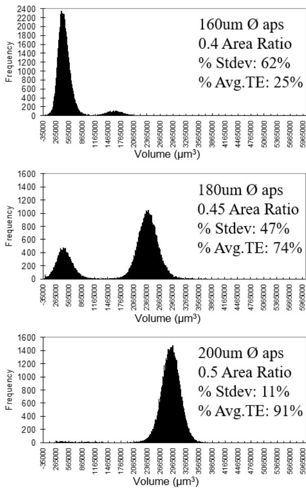
**Figure 9.** Solder paste print volume histograms per Whitmore et al.[8]
