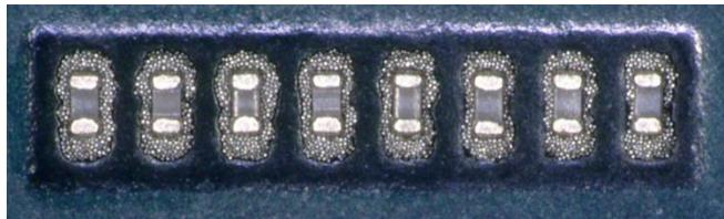
**Figure 5.** M0201 components placed in wet paste from first assembly test.
