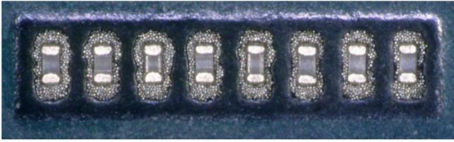
**Figure 5.** M0201 components placed in wet paste from first assembly test.
