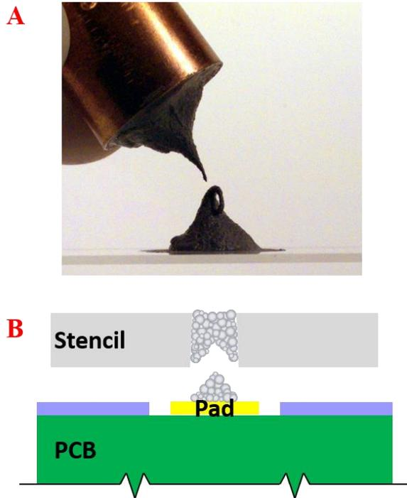
**Figure 11.** Paste release from clogged aperture; scaled up experiment A [10] and theoretical representation B.
