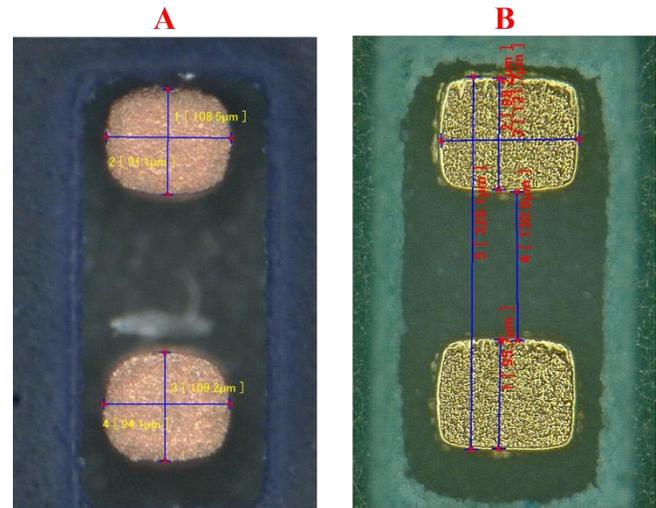
**Figure 13.** M0201 pads. A - Original board, Cu/OSP pads. B - New board, ENIG pads.
