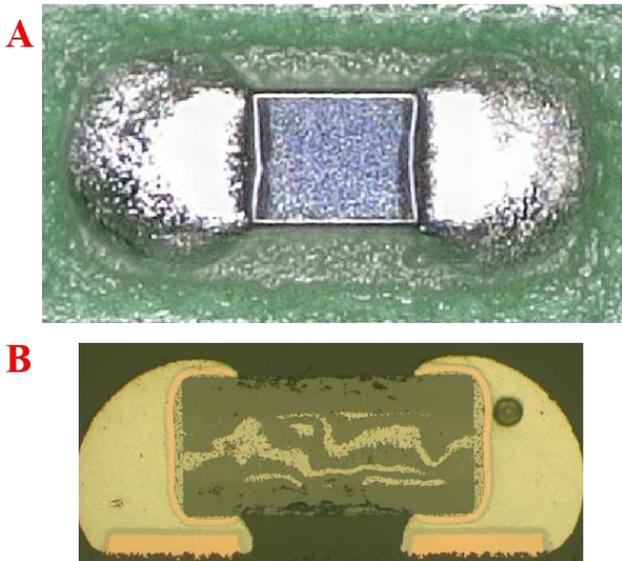
**Figure 6.** Swollen solder fillets on assembled M0201 component; top view A and cross section perspective B.
