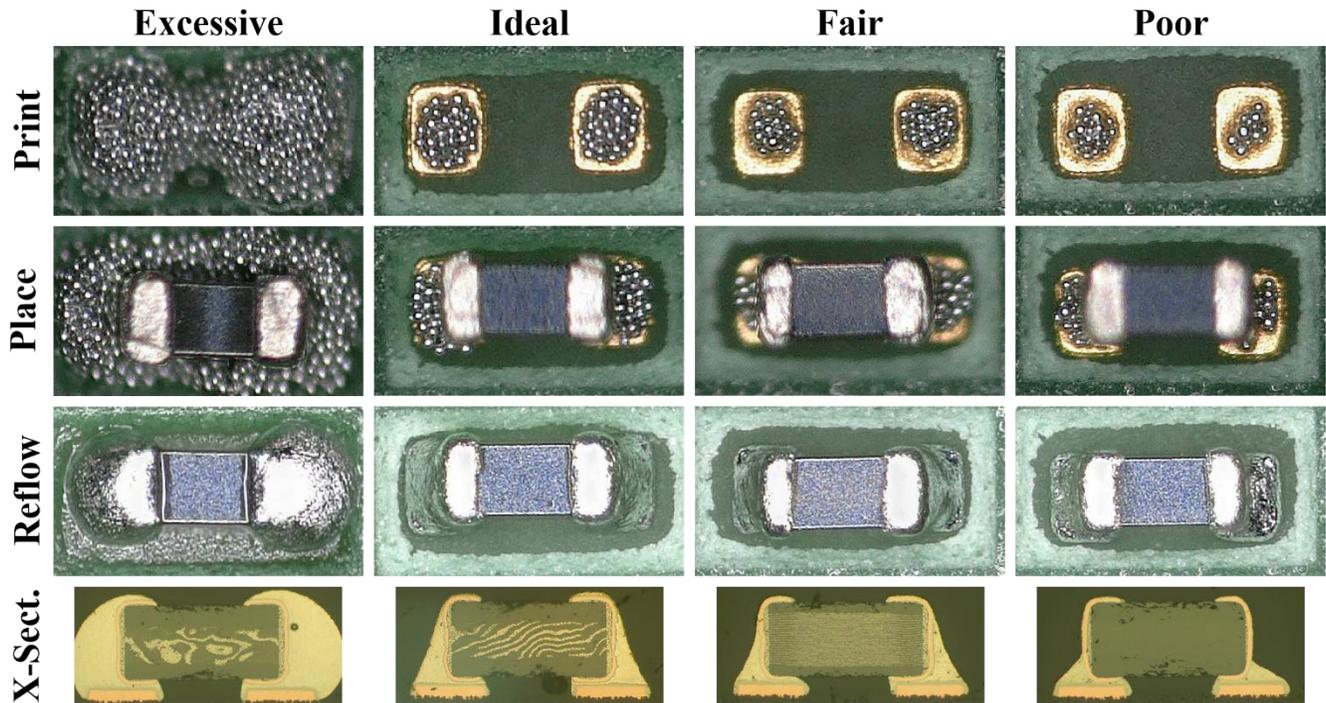
Figure 14. Example outcomes from M0201 assembly test.
