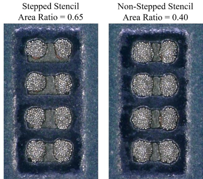
**Figure 3.** M0201 print deposits from the first assembly test comparing stepped and non-stepped stencil results.
