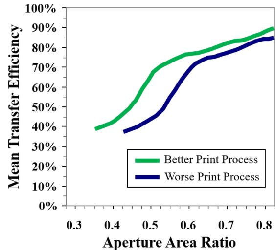
**Figure 7.** Solder paste print transfer efficiency response to aperture area ratio.
