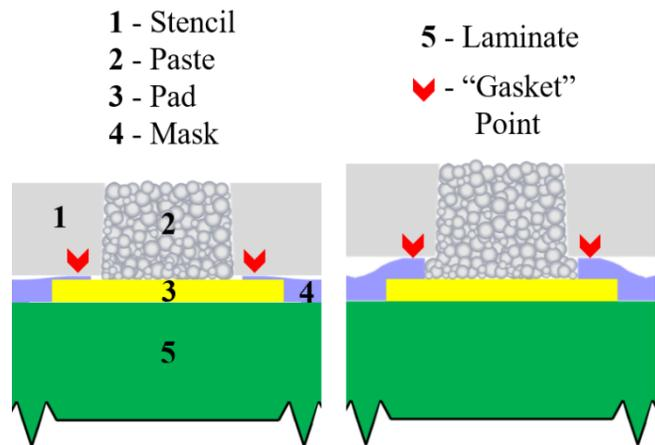
**Figure 4.** More print volume results when the stencil gasket point is further away from the pad.
