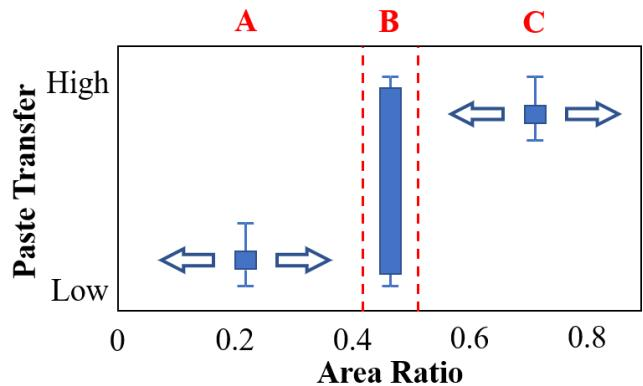
**Figure 10.** Solder paste print transfer scatter trends, simplified model.
