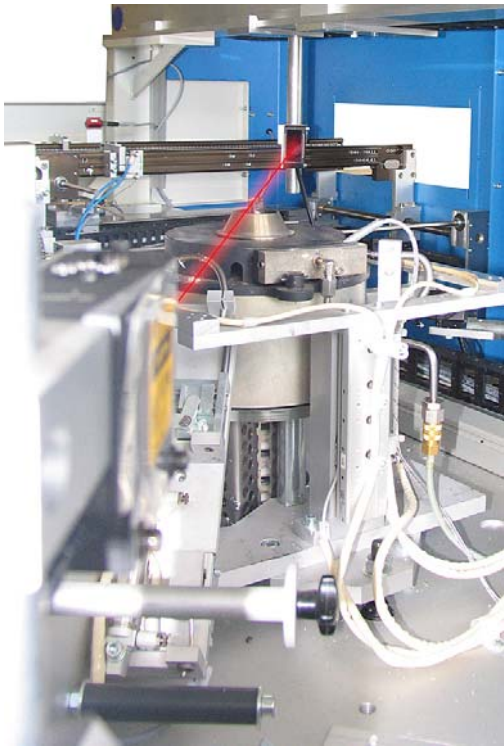
Figure 7. Laser Measuring System for Control of the Solder Wave Height
