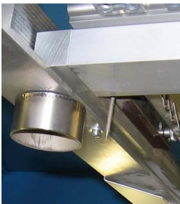
Figure 5. Measuring Needle to Control the Solder Wave Height
