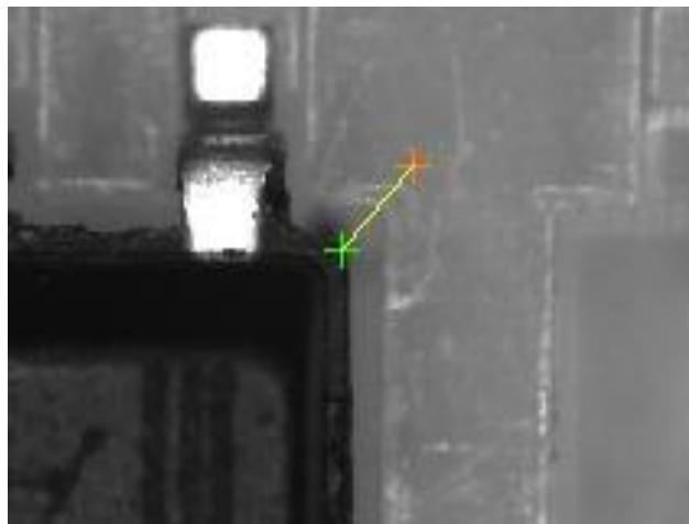
Figure 13 - The orange marker indicates the coordinates of registered fiducial point; the green marker indicates the user correction.
