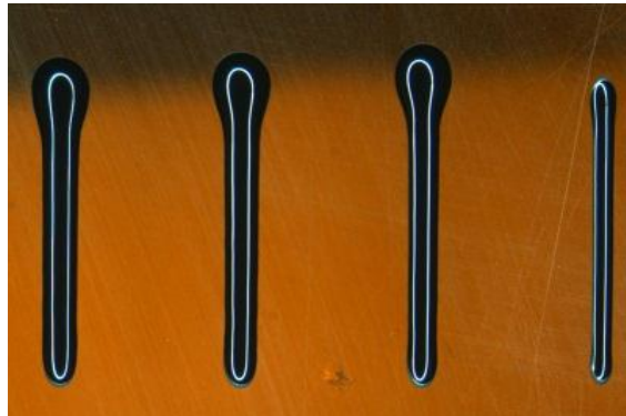
Figure 10 - Material study of only varying valve opening. Rightmost line is smallest opening
