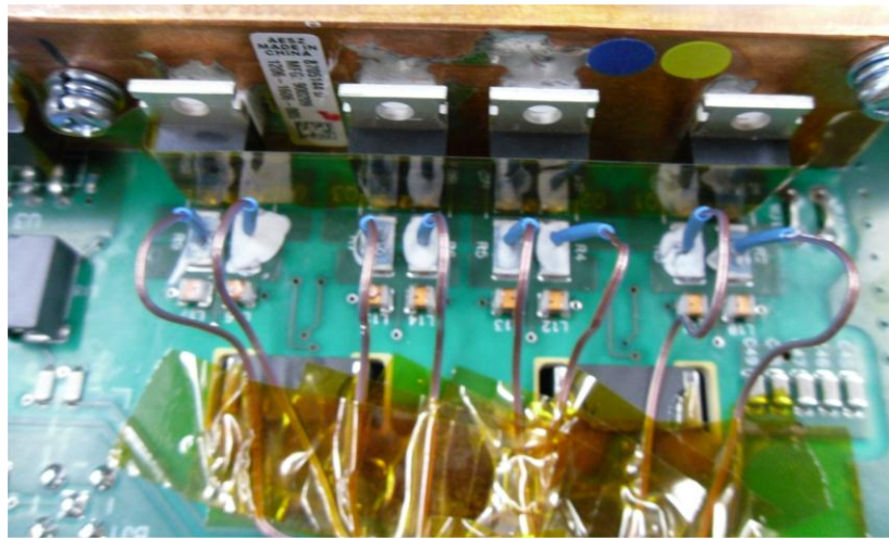
Figure 9: Thermocouple placement on Gate Drive Resistors
