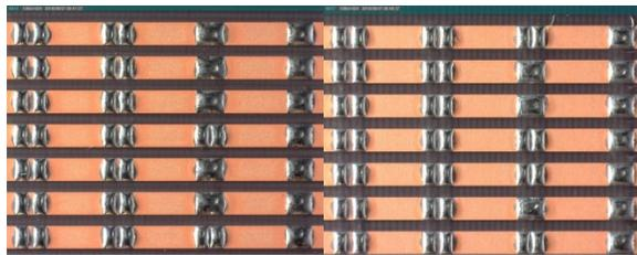
**Figure 11.** Baseline Alloy with Slow Profile (L) Fast Profile (R)
