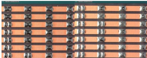
**Figure 12.** Bismuth Alloy 1 with Slow Profile (L) Fast Profile (R)
