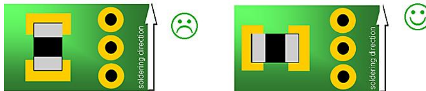
Figure 6 – Alignment of neighbouring SMD components
