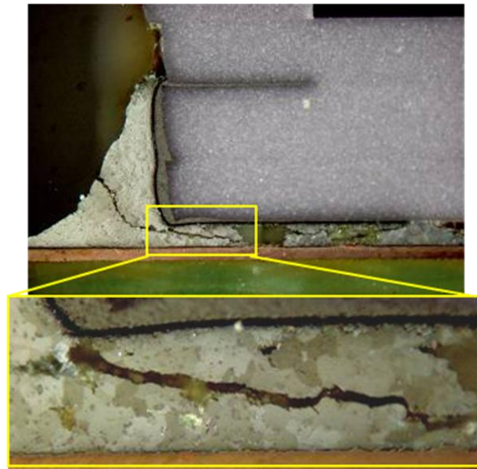
Figure 23: 5x7 Ceramic Oscillator, assembled with SAC solder, failed at 1586cycles in 0-100°C thermal cycling.
