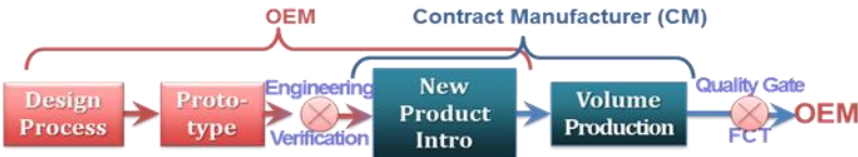
Figure 1: A typical OEM-to-CM product flow
