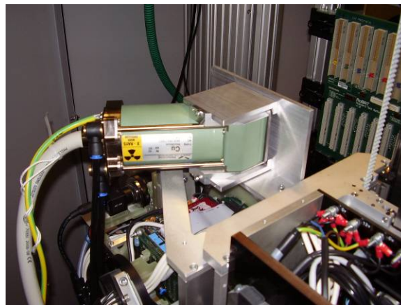
Figure 5- Source mounted in the test system
