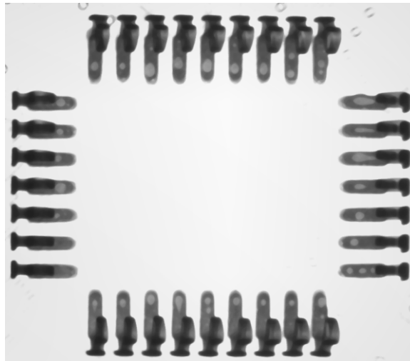
Figure 16 - Solder voids on a PLLMC surface mount IC socket
