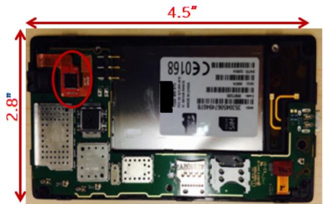
Figure 3.6. Chemical decapsulation performed on a package mounted on a flex cable while the phone stayed fully assembled
