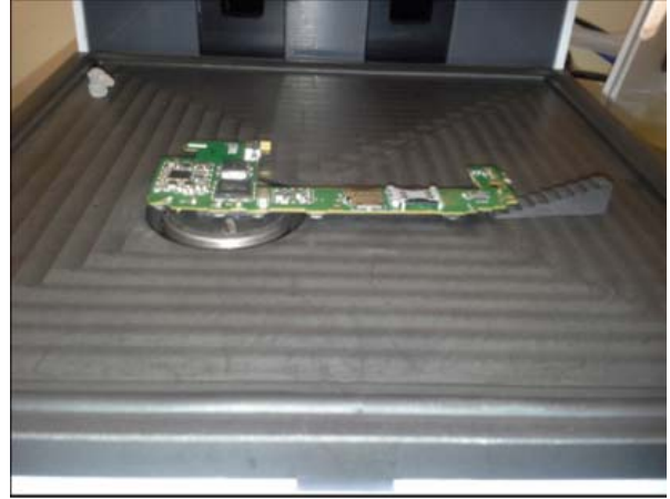
Figure 3.5. An inside view of the chamber of chemical etcher capable of accommodating a PCB from a phone board
