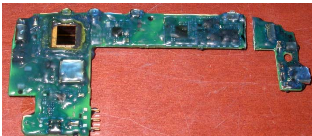
Figure 3.4. An image of a phone board that had to be cut to fit inside the conventional automated chemical etcher
