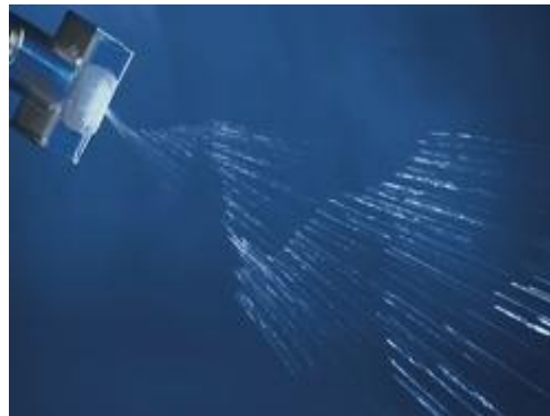
Figure 3 – Oscillating nozzle spray pattern.
