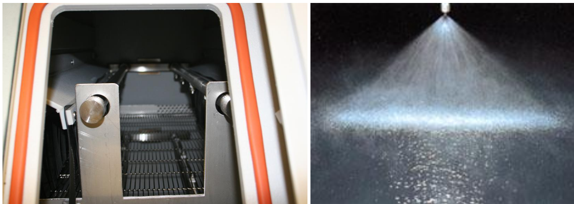
Figure 1 – Prewash with V-Jet nozzles and V-Jet spray pattern.
