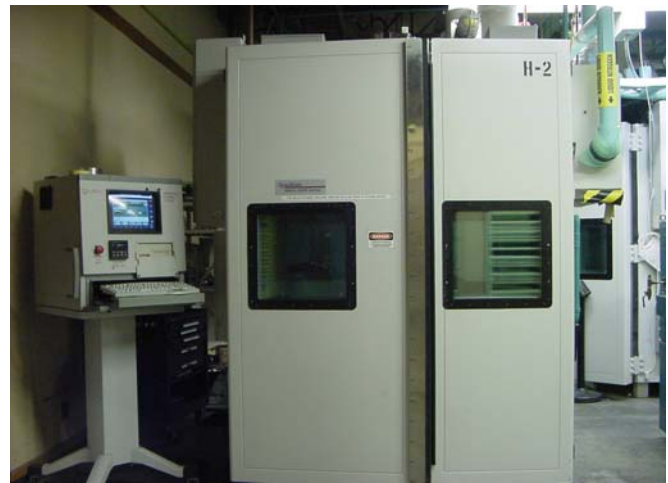
Figure 2 CET Performed in HALT/HASS Chamber
