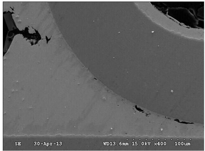
Figure 15: SEM Image of Thermal Fatigue Crack in QFP Solder Joint (SAC305 Alloy)
