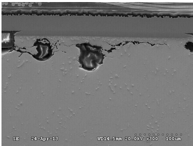
Figure 10: SEM Image of Incomplete Crack Propagating Through Solder Joint after 3000 hours ATC, near board side IMC (Sunrise Alloy)
