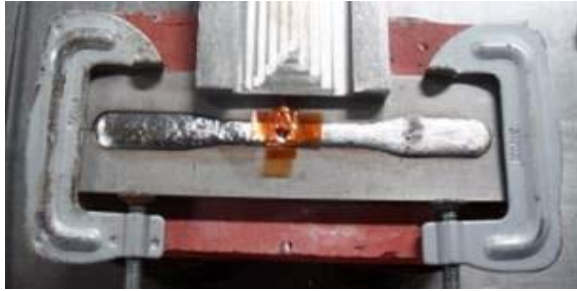
Figure 10. Set-up for casting bulk solder test pieces
