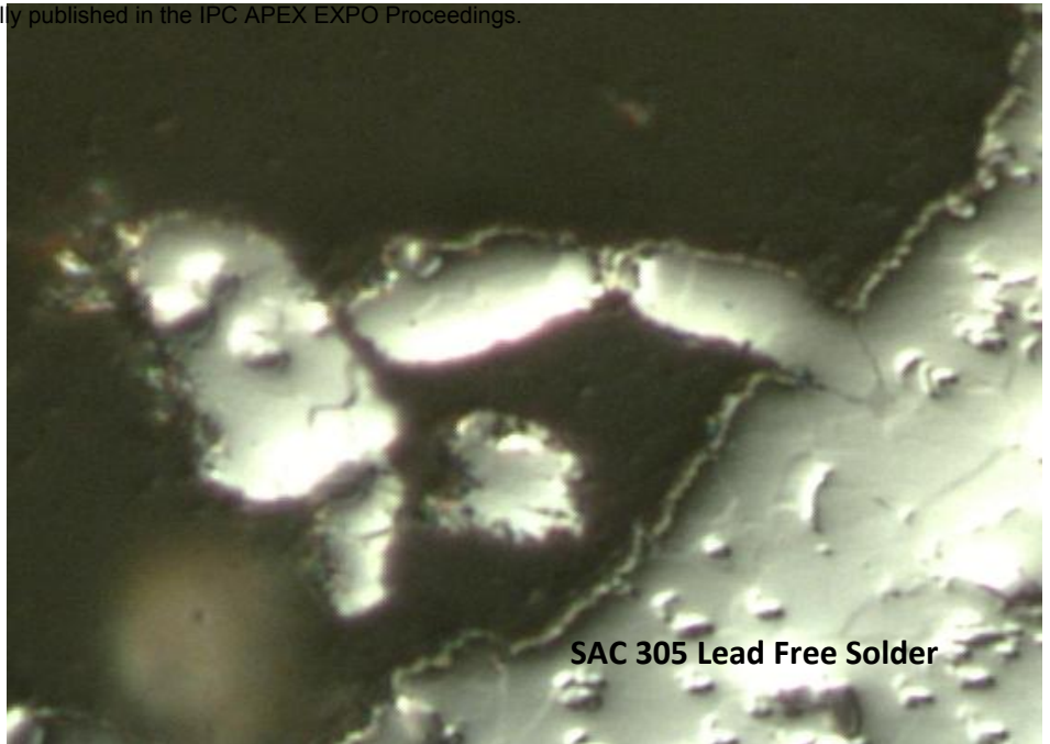
Figure 9 – Optical Image primary whisker in cross-section at 1000X
