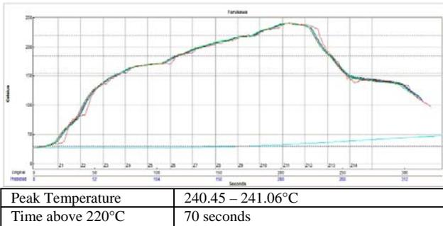
Figure 7: Reflow profile of SAC solder paste samples
