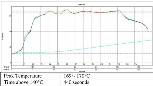
Figure 6: Reflow profile of JRP solder paste samples
