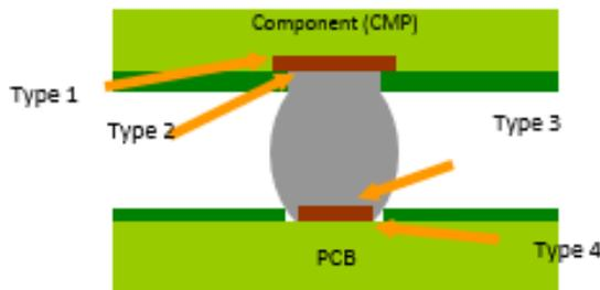
**Figure 14:** Failure disbond type categories
