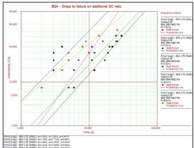
**Figure 12:** Weibull 2-P distribution of BSA leg across various monitoring daisy chain nets
