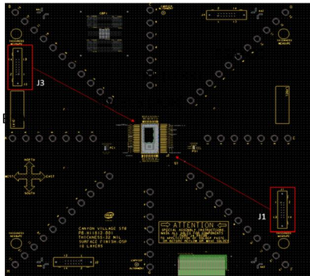
Figure 8: Top views of the printed circuit board used for the Mechanical Shock tests.
