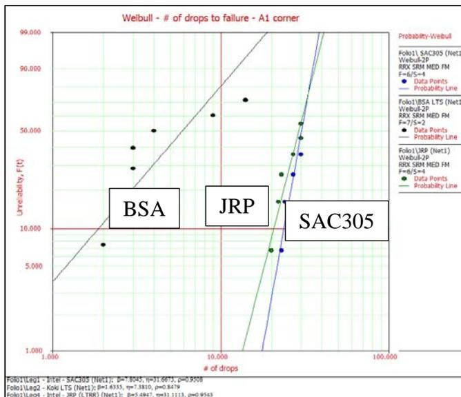
**Figure 10:** Weibull 2-P distribution of Net A1 comparing SAC305, BSA and JRP
