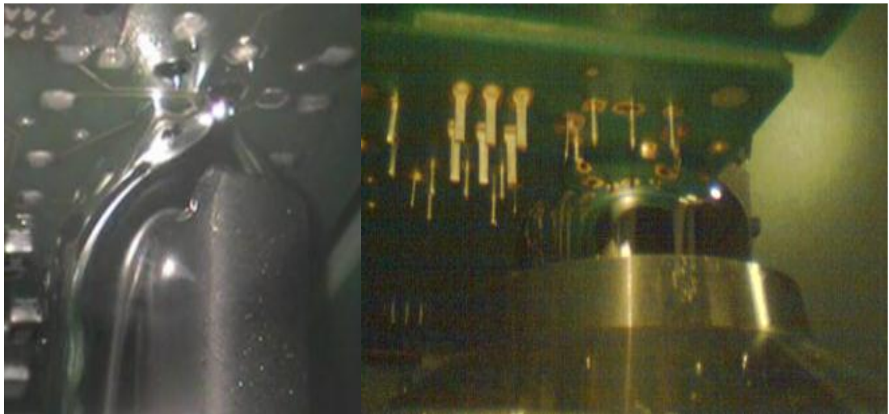
Figure 2: Solder fountain with “non-wetted” nozzle (left) and “wetted” nozzle (right). Photo courtesy of JUKI.
