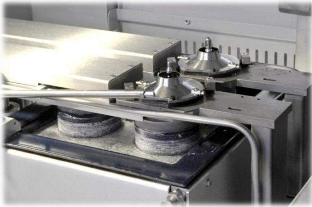
Figure 4: Dual solder fountains on X-Y axes; 1.8mm (left) and 4mm (right). Photo courtesy of JUKI.
