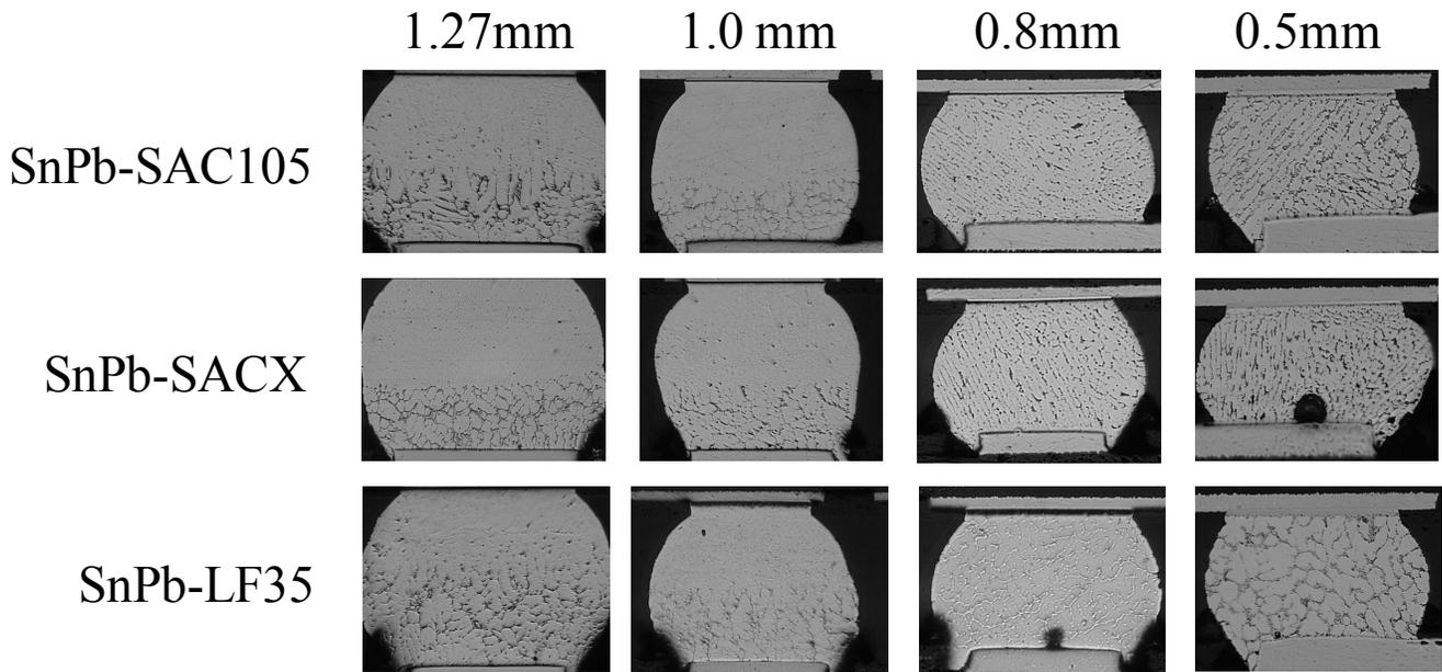
**Figure 2 – Typical microstructures for mixed SnPb/Pb-free solder joints tested in this study. Such joints were reflowed at peak temperatures of 215 °C to produce partial mixing on the larger packages (joints shown were formed in phase 1B [4]).**
