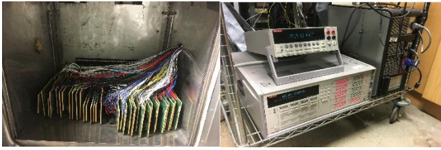
Figure 3 Test boards stacked inside the chamber (left); Multimeter and multiplexer monitoring system.
