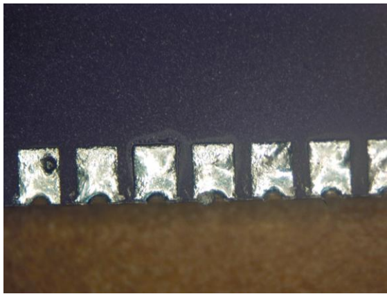
Figure 4a: Fail - Flux residue detected at 40X
