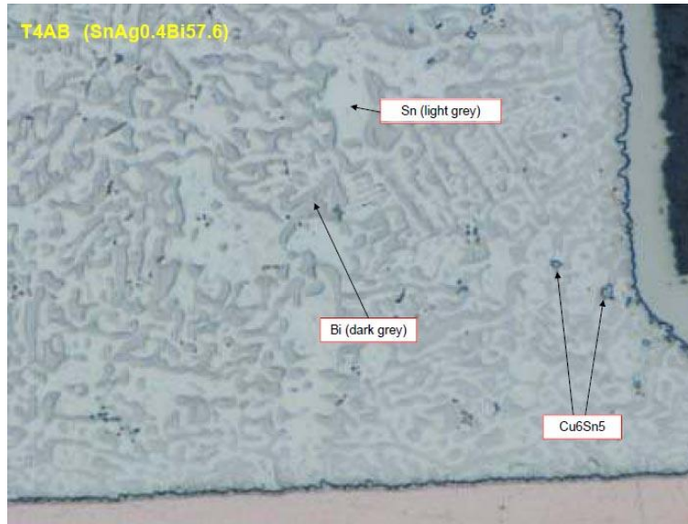
Figure 28: Sn57.6Bi0.4Ag soldered 3216[1206] chip component cross-section.
