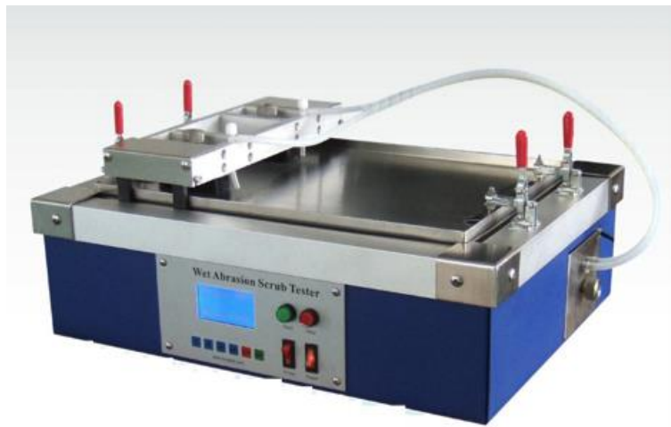
Figure 3: Wet Scrub Tester
