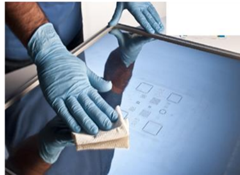
Figure 1: FPN and Phosphonate Nano-Coatings on Stencils
