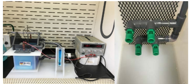
Figure 2. Test cell 8 L with educator flow and knife agitation.
