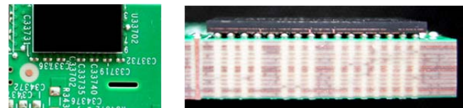
Figure 5. Memory device polished to the edge row to be used for reflow simulator
