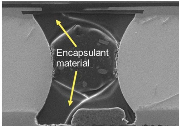
**Figure 11.** Post-SMT coverage of edge solder joints after further optimization of dip process
