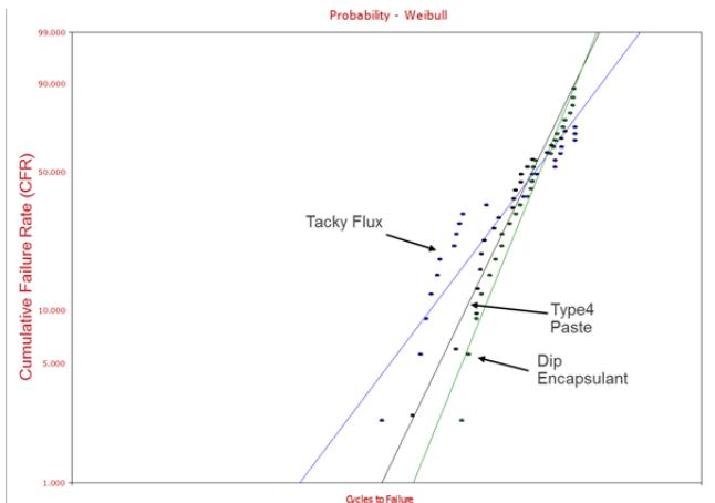
Figure 15. Example Weibull plot illustrating improvement in corner joint reliability with encapsulant flux, but reduction in reliability with tacky flux.
