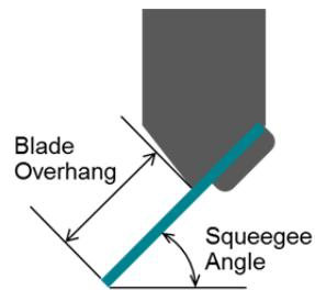
**Figure 3.** Illustration of squeegee blade for angle and overhang reference.
