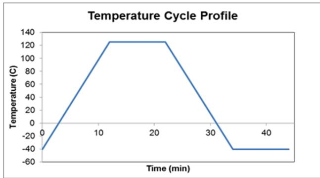
Figure 14. -40/125°C temperature cycle profile
