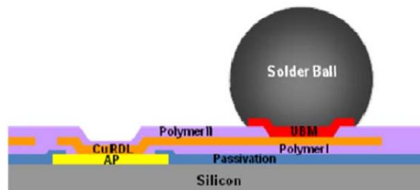
**Figure 1.** RDL Type Wafer Level Package
