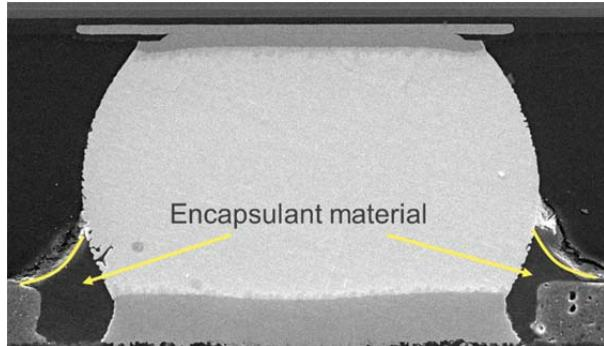
**Figure 9.** Post-SMT coverage is limited to the bottom of the solder joint with no reinforcement near the package UBM
