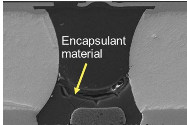
**Figure 13.** Post-SMT encapsulant coverage after printing the material using paste-print parameters. Only the bottom of the solder joint is reinforced.
