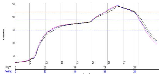
**Figure 2.** Standard lead-free reflow profile with 245°C peak.
