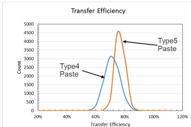
**Figure 5.** Transfer Efficiency histogram for Type 4 and Type 5 solder paste on a 100 $\mu\text{m}$  thick stencil with 220 $\mu\text{m}$  aperture (0.55 AR). Type 4 Cpk = 1.22; Type 5 Cpk = 2.52.
