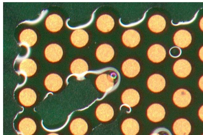
**Figure 12.** Print result of the encapsulant flux. The material flows across multiple pads.
