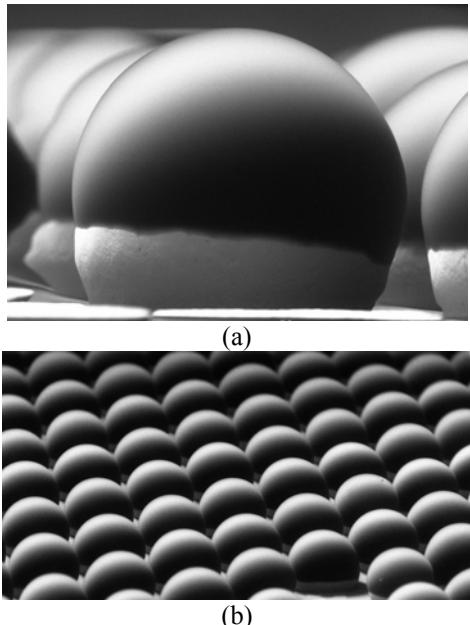
**Figure 8.** Encapsulant coverage on solder balls after dipping. (a) Single solder ball showing approximately 75% coverage by wetted height; (b) Array of balls showing consistency in coverage.
