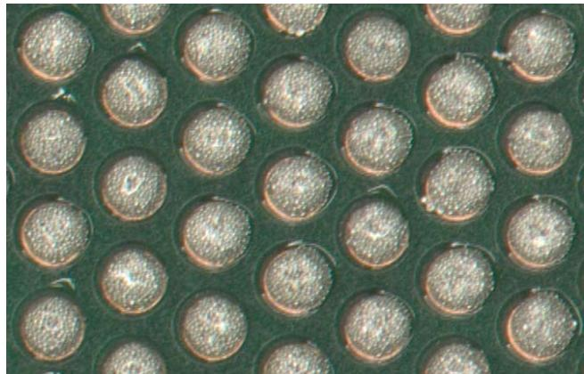
**Figure 6.** Print quality using Type 5 solder paste
