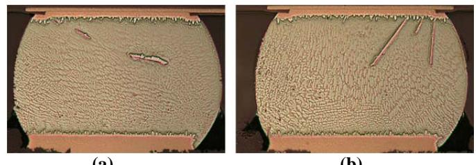
**Figure 7.** Cross-section images for assemblies built with different solder paste. (a) Type 4 paste; (b) Type 5 paste.
