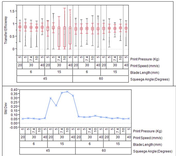
**Figure 4.** Print results as a function of Pressure, Speed, Blade Length and Squeegee Angle. Top: transfer efficiency; Bottom: standard deviation.
