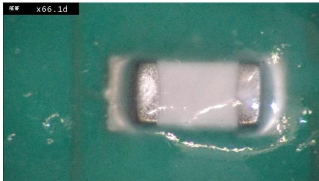
**Fig 17.** SR coated discrete showing no evidence of corrosion.
