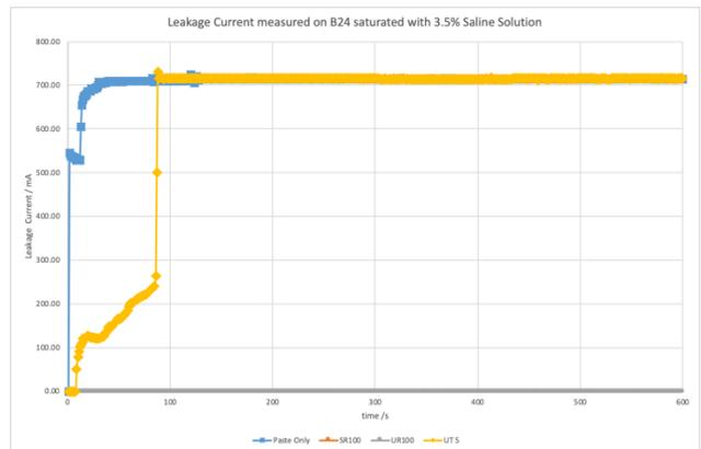
**Fig 3.** leakage current measurements for different coatings and thicknesses.
