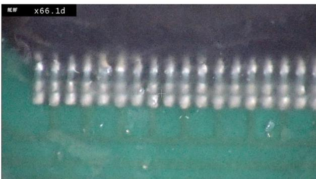
**Fig 13.** UR coated QFP under white light – no evidence of corrosion.
