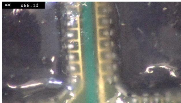
**Fig 15.** UR Coated QFN showing no evidence of corrosion
