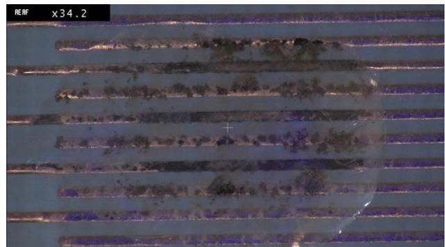
**Fig 4.** corrosion products forming on no-clean solder paste after 30 seconds powered with saline saturation
