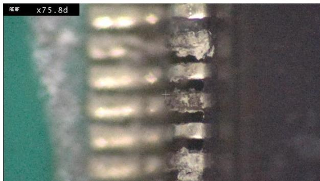
**Fig 10.** Corrosion evident on AR coated QFP leads
