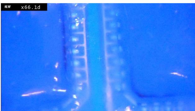
**Fig 14.** UR Coated QFN under black-light showing coverage
