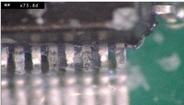
**Fig 11.** Corrosion evident on and between AR coated QFP leads.
