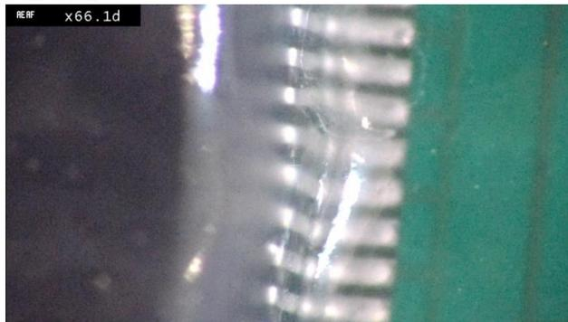
**Fig 16.** SR coated QFP lead showing no evidence of corrosion.
