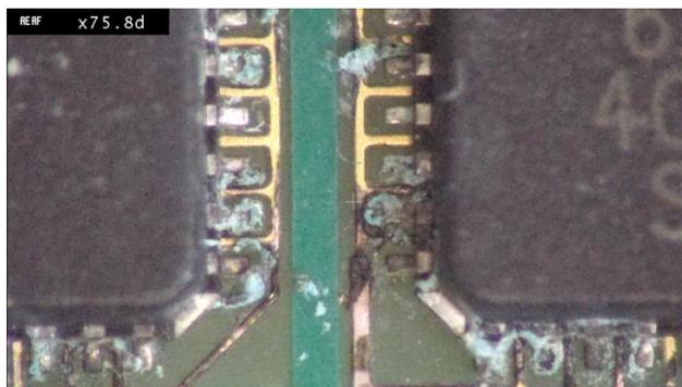
**Fig 7.** Corrosion of UT coated QFN array
