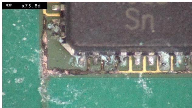
**Fig 6.** corrosion of UT coated QFN.
