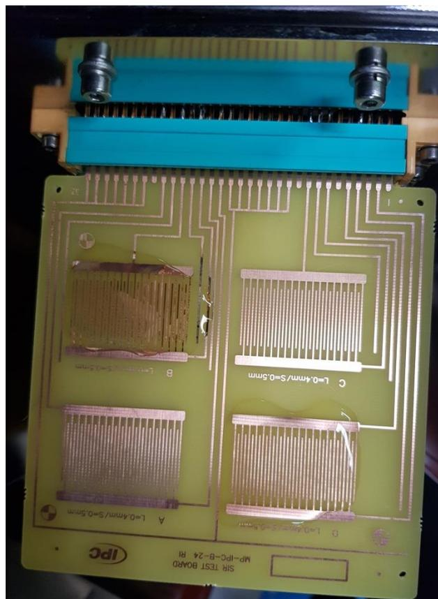
**Fig 2.** IPC-B24 coupon mounted horizontally in SIR test rack.
