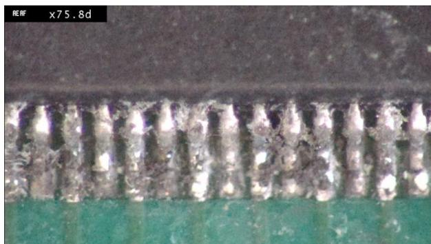
**Fig 8.** Corrosion of UT coated QFP leads
