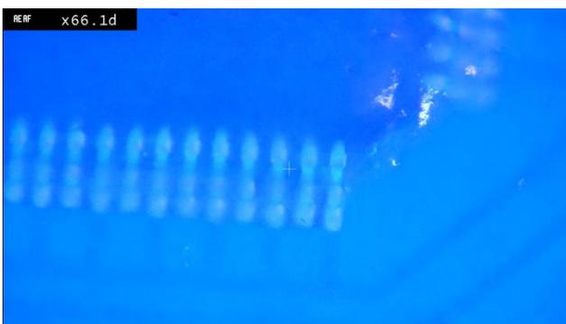
**Fig 12.** UR coated QFP leads under blacklight showing coverage.
