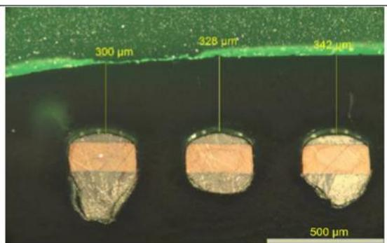
**Fig 18.** UR coverage of QFP lead down through plane of lead
