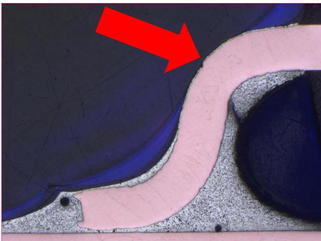
**Fig 1.** Cross-section of QFP lead showing negligible coating coverage on knee bend.
