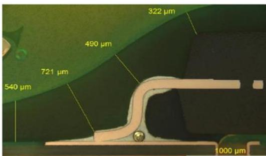
**Fig 19.** UR coverage of QFP lead
