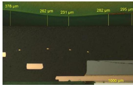
**Fig 20.** UR coverage of QFP package
