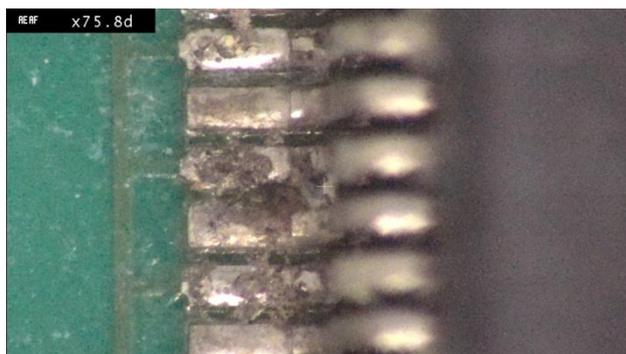
**Fig 9.** Corrosion evident on AR coated QFP leads
