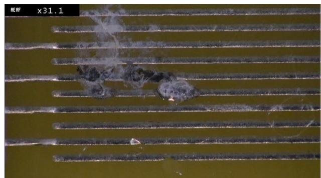
**Fig 5.** corrosion products forming on UT-5 micron after 30 seconds powered with saline saturation
