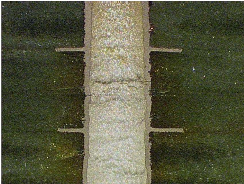
Figure 5: Microsection of via with failure in region where non-functional pads have been retained.
