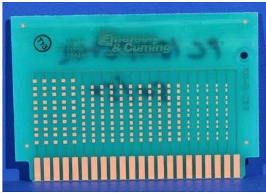
Figure 2. Printed circuit board coupon 101 mm x 69 mm x 1.2 mm thick.
