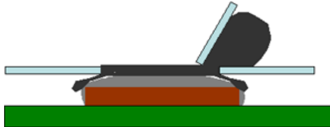
Figure 4. Paste bleed due to problem of stencil gasketing on non-planar HASL coating
