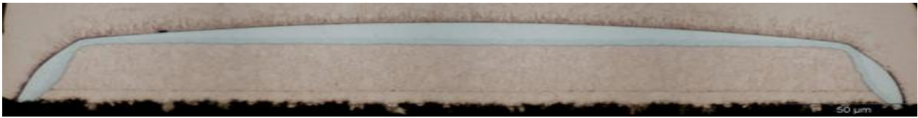
Figure 7. Cross-section of an ideal HASL finish
