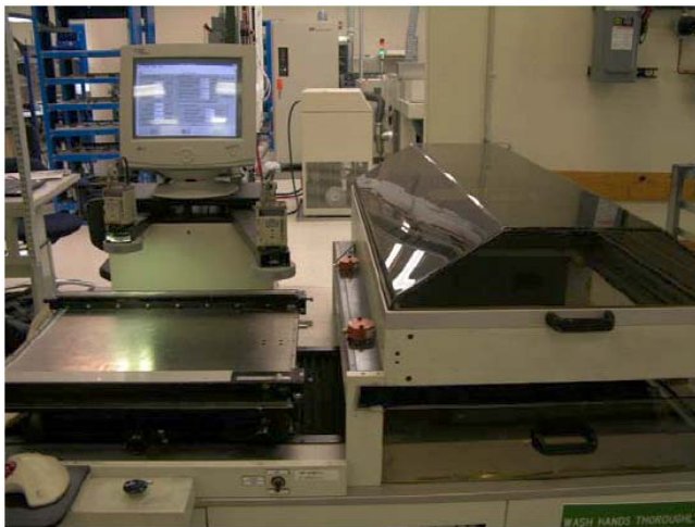
Figure 6: Solder paste screen tool modified for connector site screening
