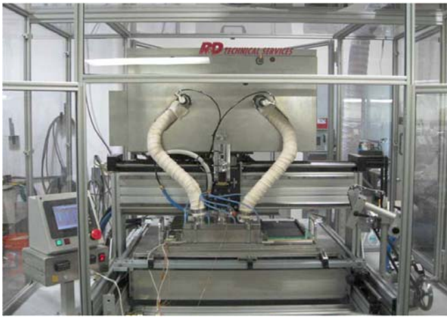
Figure 2: Local vapor phase machine for large surface mount connector rework
