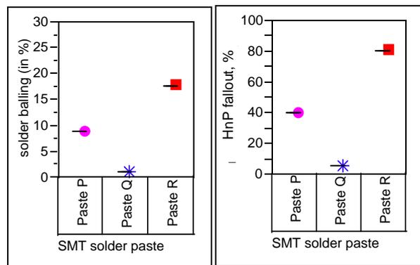
**Figure 24:** Higher solder balling % shows higher HnP fallout rate.
