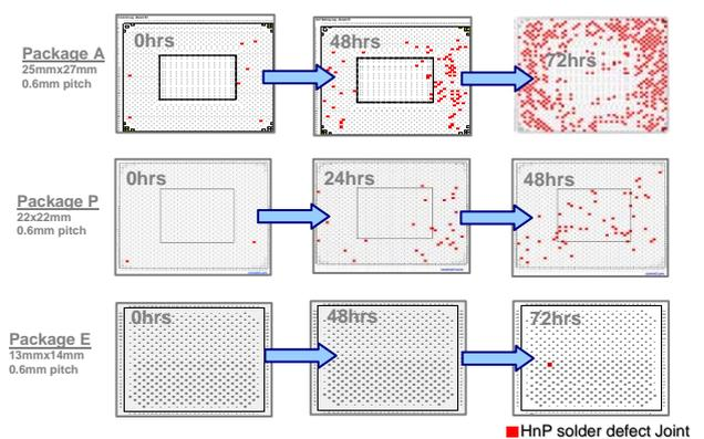
**Figure 27.** Impact of baking time in air on the propensity to form HnP defects after reflow soldering for three different BGA packages
