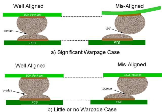
Figure 10. A scenario where significant warpage of the component and board can lead to Mis-placement of the component causing an HnP defect
