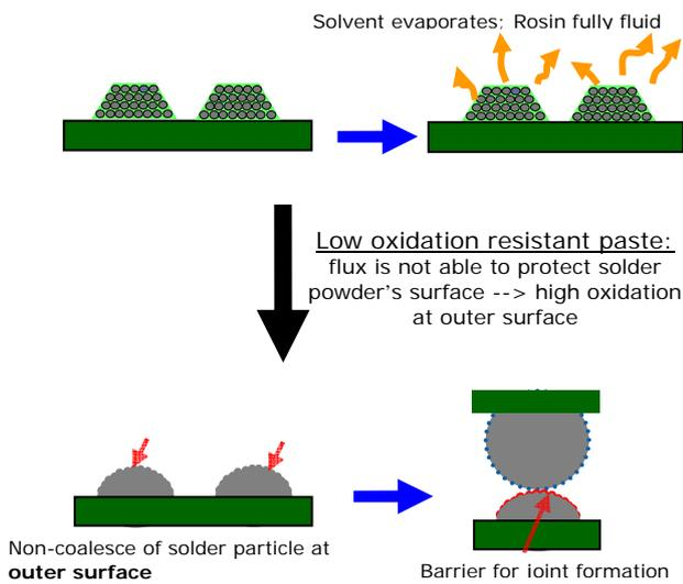
**Figure 25:** Mechanism of Oxidation resistance affecting HnP.
