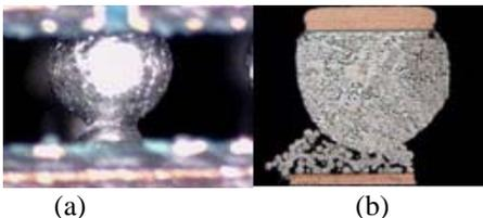
Figure 11. Incomplete reflow HnP defect
