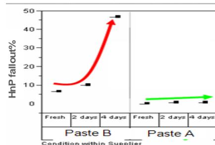
Figure 21: Comparison between solder paste A and B at 29°C for 4 days, changes in viscosity & pH recorded together with HnP fallout
