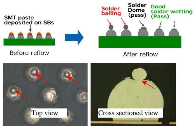
**Figure 23:** Wetting test on solder balls and solder balling images.
