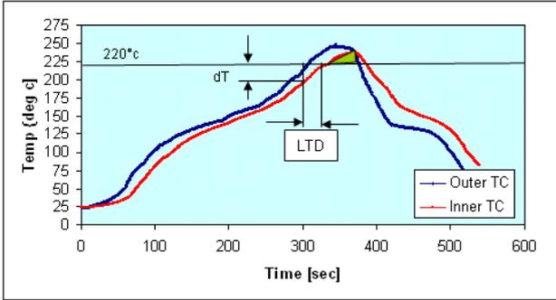
Figure 14. BGA liquidus time delay
