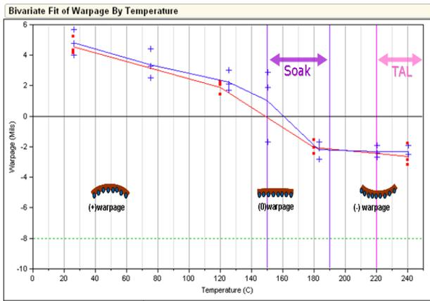
Figure 33. BGA warpage during reflow
