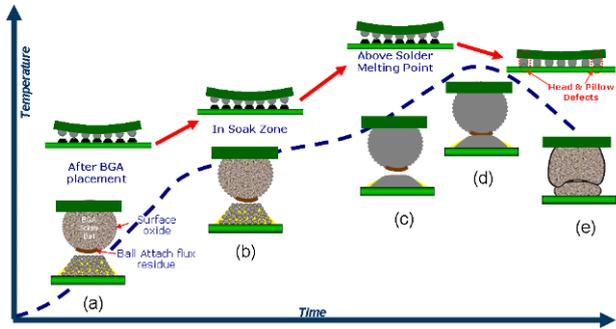
**Figure 2.** Depiction of the Head - and - Pillow Defect Formation Mechanism.
