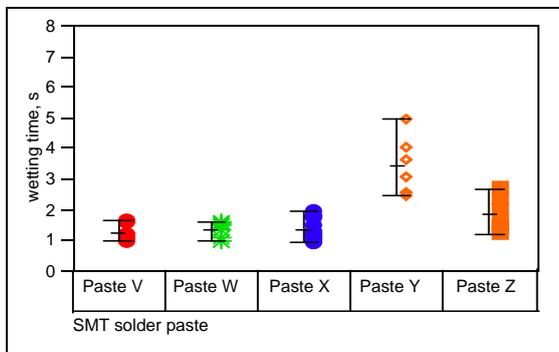
**Figure 22:** Wetting time results for multiple solder pastes using a wetting tester
