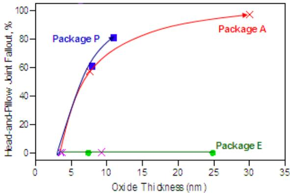
**Figure 28.** Variation of HnP Solder Joint Fallout rate with Oxide thickness on the solder balls for three different BGA packages
