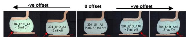
Figure 9. Optical Microscope photo-graphs of cross-sections for the misplaced BGA sockets on a test vehicle board. The off-sets for the various sockets are shown in the photos.
