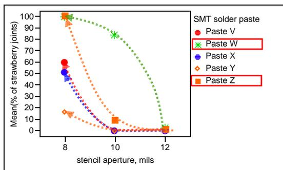
**Figure 26a:** % of non-coalesce solder paste with decreasing stencil aperture.
