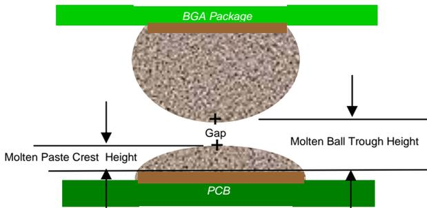
**Figure 3.** Illustration of the gap between the solder ball and the solder paste that precedes the formation of most HnP BGA solder joint defects.
