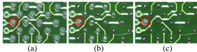
Figure 42. Paste melting delay
