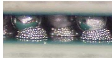
**Figure 4.** BGA balls and paste contact
