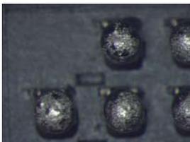
Figure 19. Dark patches on balls
