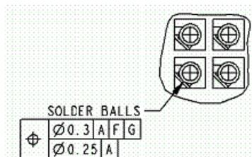
Figure 36. Typical call-out for solder ball true position in a mechanical drawing for a BGA socket.
