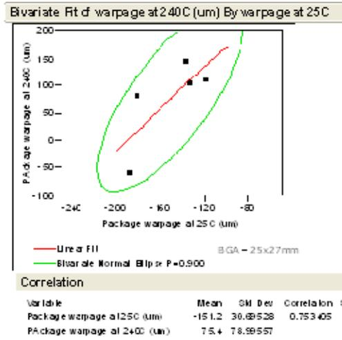
Figure 35. Warpage correlation between room & reflow temperature
