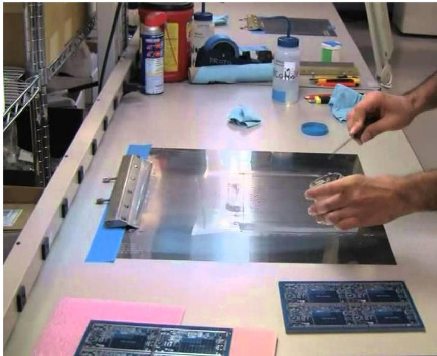
**Figure 4 – Typical manual stencil printing set- up**
