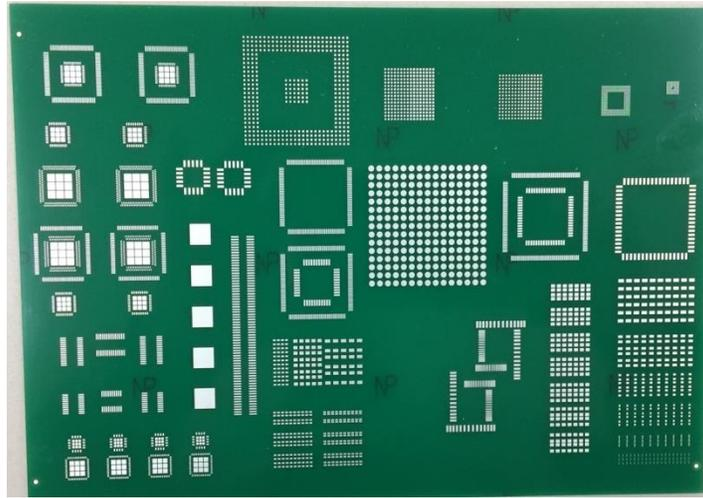
**Figure 2: Test Vehicle for Solder Paste Printing Study**
