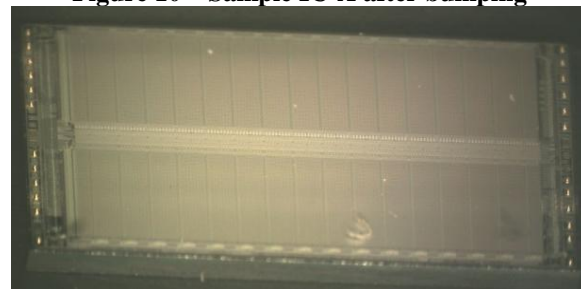
Figure 7- IC-B after bumping
