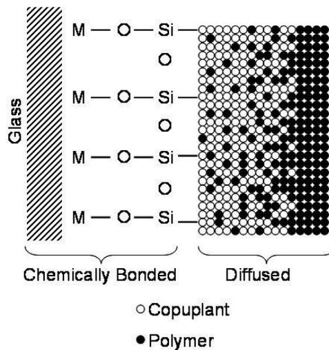
Figure 4 Schematic for conventional interdiffusion and IPN [10]
