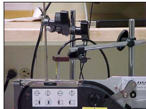
Picture 4 Blister on a feeder with ESDS, electrostatic voltage measured with a small field sensor
