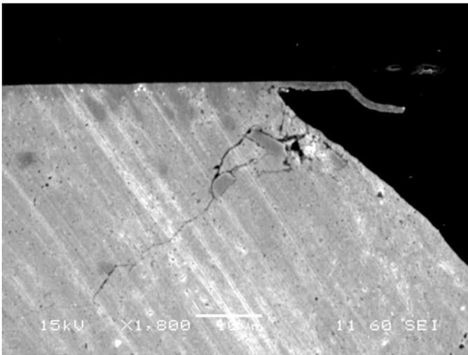
**Figure 6.** Solder joint cracking on WLCSP devices.
