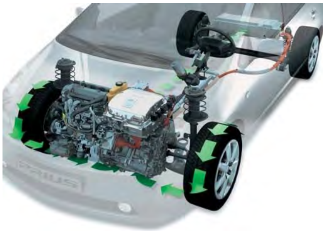
Figure 9. Regenerative brakes recapture energy normally lost when slowing down by using the traction motors as a generator.
