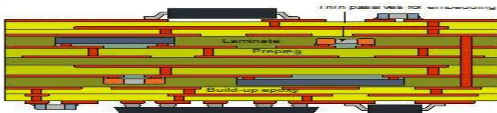
**Figure 1- Embedded component PCB**
