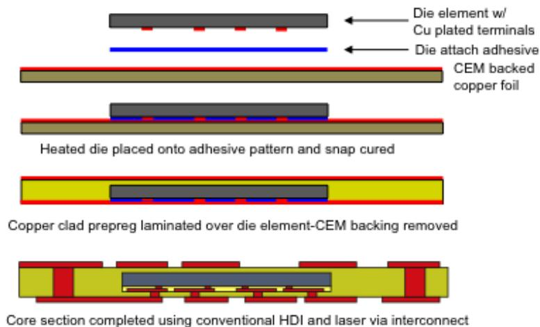
**Figure 11- Embedded core fabrication sequence**
