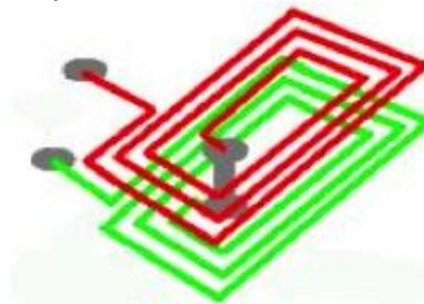
**Figure 5- Two level spiral inductor configuration**
