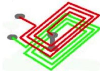
**Figure 5- Two level spiral inductor configuration**
