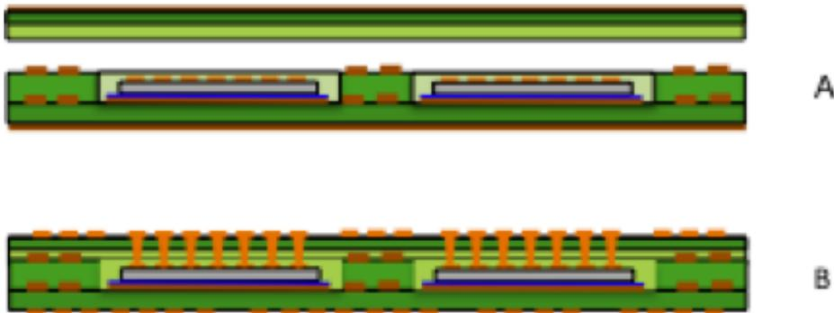
**Figure 10- Face-up, in-cavity die attach for micro-via interface**
