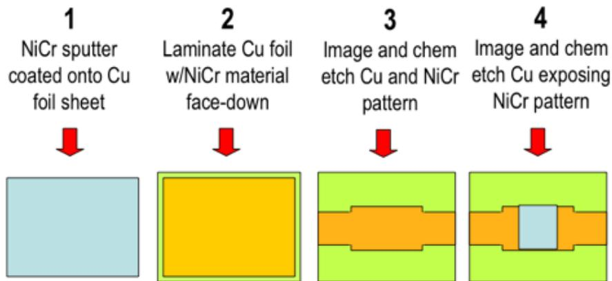
**Figure 3- Thin-film resistor process sequence**
