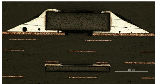
Figure 6 - EC and SMD 0402s vary in z-axis dimension
