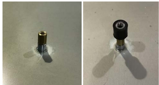
Figure 12. Metal vs rubber standoff
