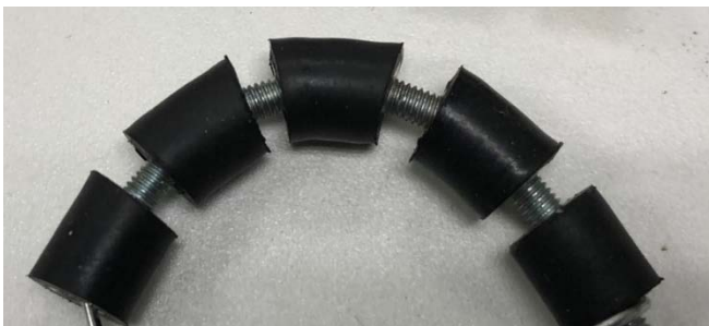
Figure 2. Rubber standoffs with excellent flexibility
