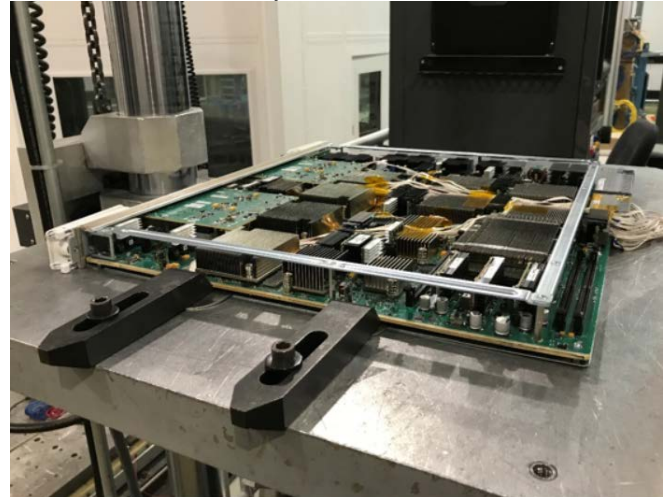
Figure 10. Product-level shock test setup
