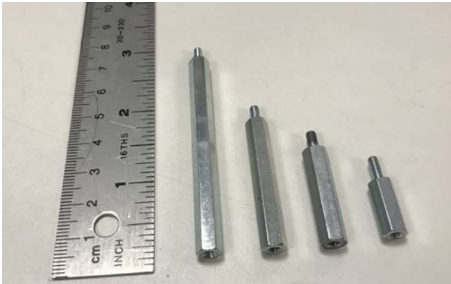
Figure 1. Typical metal standoffs used for PCBA assemblies
