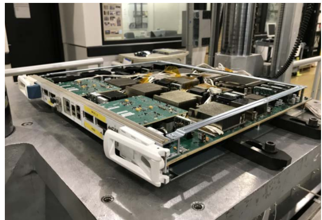
Figure 11. System tested with rubber standoffs
